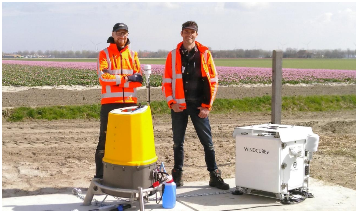
Figure 2: Samples of LiDARs, ready for verification testing at a 120 m tall mast in The Netherlands. Left: ZX300M, right a WindCube V2.1M (both offshore versions). Photo: courtesy of Pondera/Haskoning.
