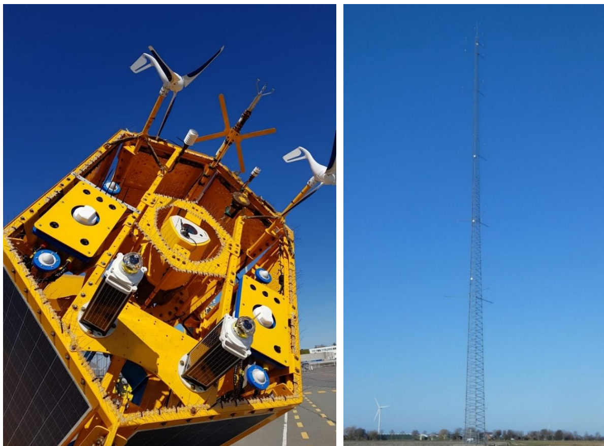
Figure 3: Left: the 'inside' of an RPS floating LiDAR prior to deployment in The Netherlands. Clearly visible is the ZX300 LiDAR in the centre of the picture. Right: the traditional way of measuring the wind, using a tall mast or tower. Photos: Author and Pondera/Haskoning.
